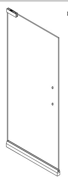
PL424 - 2 X 6½" EURO TOP PATCH (CLAD) BY P.R.L. GLASS ½" CLEAR TEMPERED GLASS BY P.R.L. GLASS PL-150DS BTM RAIL (CLAD) BY P.R.L. GLASS
