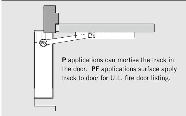
**P** applications can mortise the track in the door. **PF** applications surface apply track to door for U.L. fire door listing.
