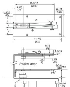
Extended spindles available in 1/2"(13mm) increments up to 2"(51mm)
