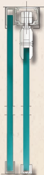
Top Hung Slider Door/Sidelite 2 3/8" Diameter Roller
